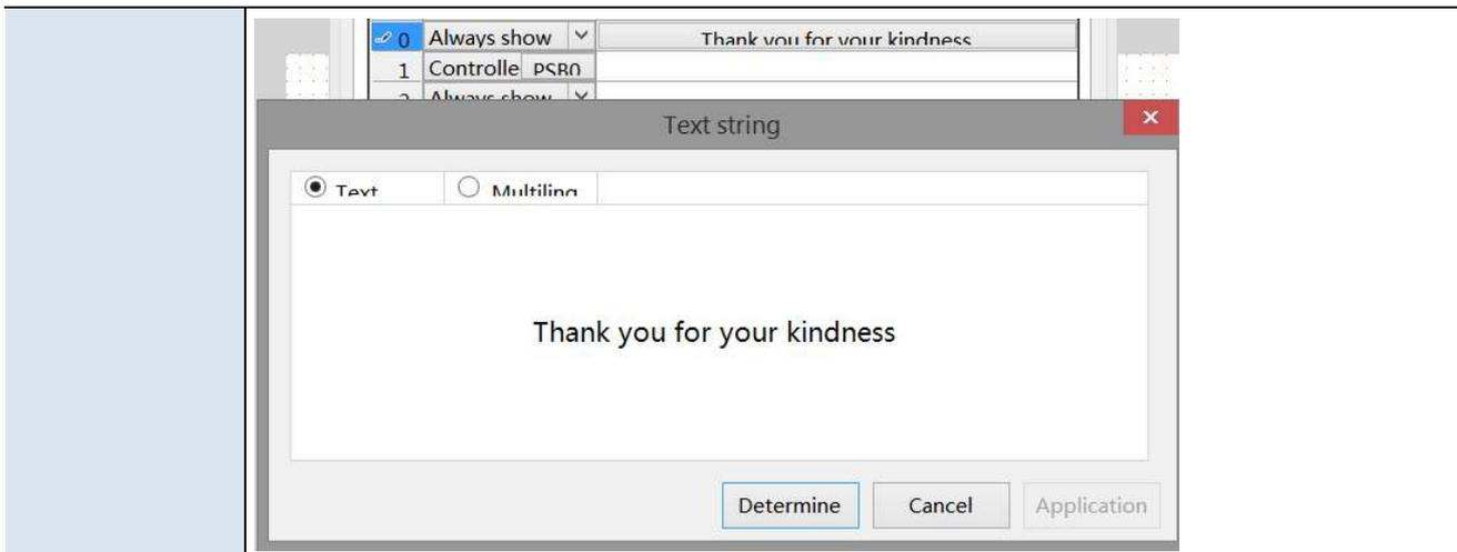
controlled by coil To set the address of the triggering coil first, then right-click and select the item to be displayed in the displayed content
