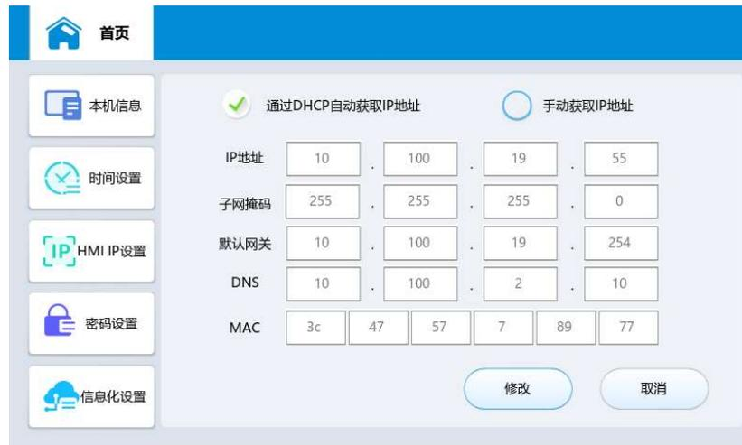
Under the condition of manually setting the IP address, after changing the IP address, click "OK" to save, and the page will pop up with the modification result; If you click the "Cancel" button, the modified content will not be saved.
