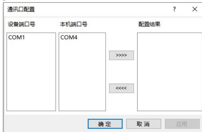
10. At this point, it is necessary to configure the port and connect the device port with the local port. First, click to select the device port number, then click to select the local port number, and then click the middle button. The configuration result will be displayed on the right side.
