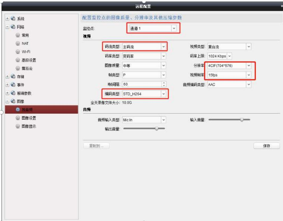
5. Based on all the configuration information, it can be concluded that the RTSP address of the Ezviz camera used in this example is `rtsp://admin:KPEBID@10.100.19.214:554/h264/ch1/main/av` stream. You can directly input this address into the camera playback control for monitoring.
