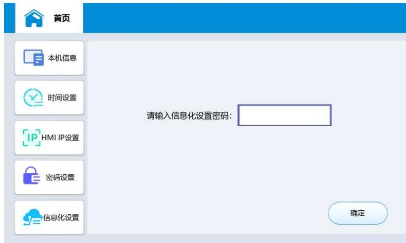
After successfully entering the password, you can enter the relevant information configuration page. The homepage allows you to view information related to information technology, such as the current device's networking method, signal strength, SIM card status, and remote related flag status.
